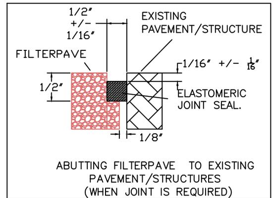
ABUTTING FILTERPAVE TO EXISTING PAVEMENT/STRUCTURES (WHEN JOINT IS REQUIRED)
